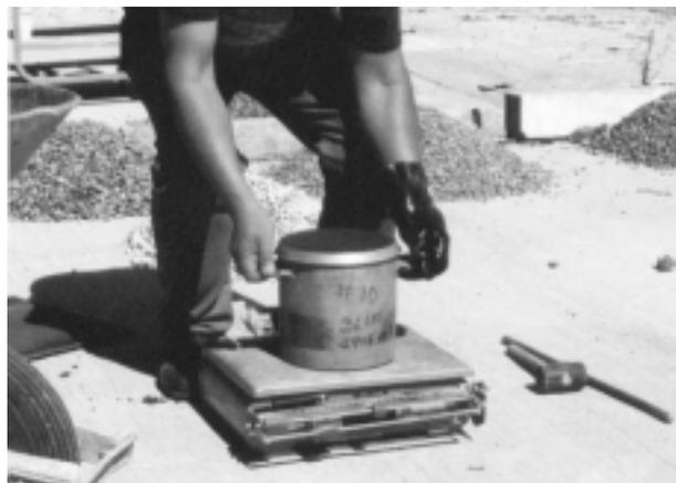
*Figure 3-6: The unit weight test is the primary test that should be used to solve yield problems.*
